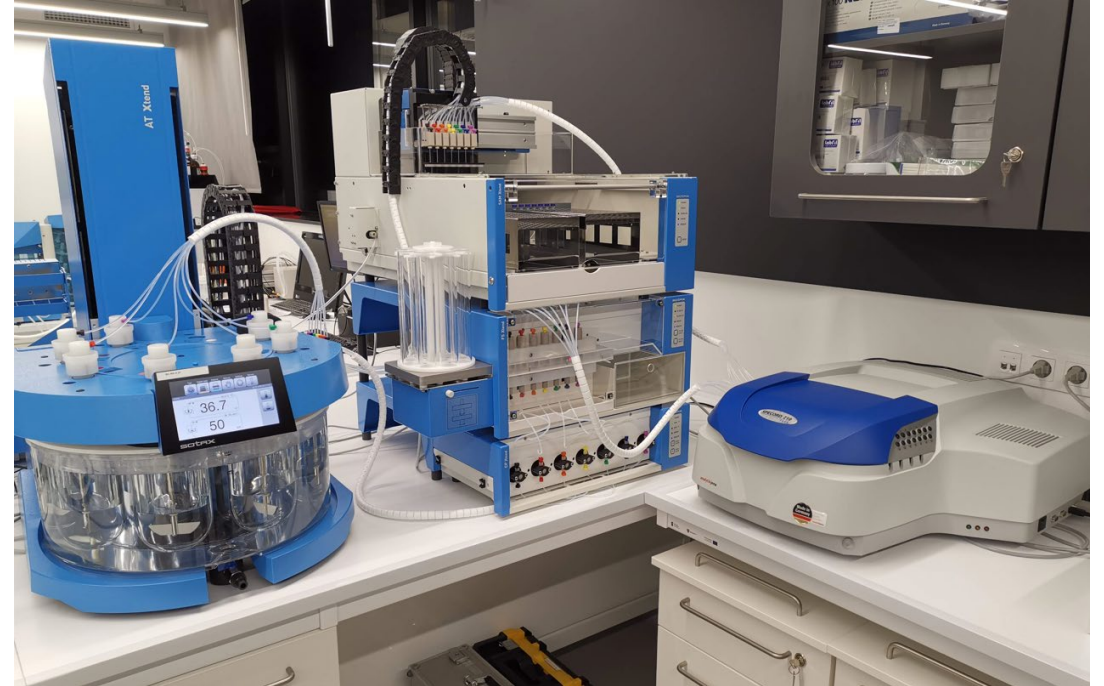
Semi-automatic SOTAX Xtend system for release testing using basket/paddle/paddle over disc/mini-vessels & mini- paddles/immersion cells in on/off-line configuration, consisting of: ATS Xtend apparatus equipped with Hollow- Shaft, Return Line and Media Replacement systems, CP pump, FS filtration station, SAM S fraction collector and UV- Vis spectrophotometer.
