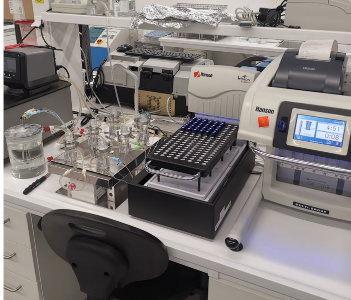
Teledyne Hanson Research automated Vision Microette System with a set of vertical Franz diffusion cells for testing the release and permeation of API from liquid and semi-solid dosage forms.
